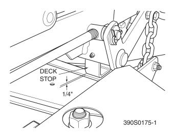
Figure 6-8. Cutter Deck Stop
